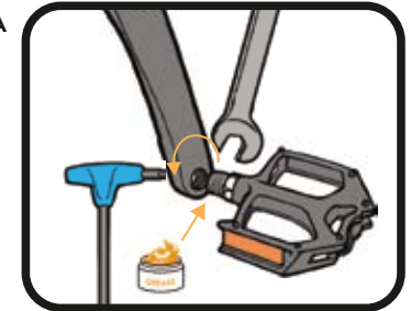
L Non-driveside tightens counter-clockwise
